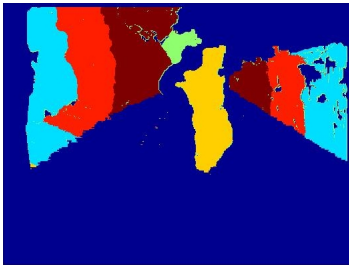
(b) Clustering the disparity value using the mean shift algorithm
