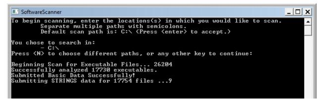
Figure 1 SoftwareScanner in action. Note that the scan found 26,204 files, but only analyzed 17,730 of them. That means there were 8,474 duplicate executables on this computer.
