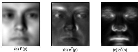
Fig. 7. Mean and variance maps used. (a) Ensemble mean of albedo, (b) Ensemble variance of albedo, (c) Error variance of the surface normal.
