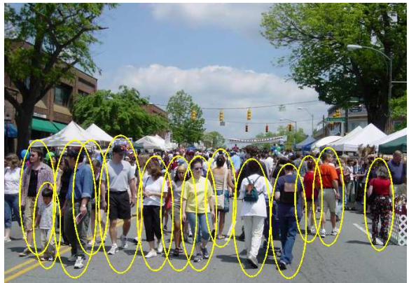
Figure 1. Image demonstrating the performance of our system in a complex scene. The image ( 689 \times 480 pixels) is scanned at 10 scales to search for humans of multiple sizes. We achieve minimal false alarms even though the number of detection windows is 44,996 (best visualized in color).
