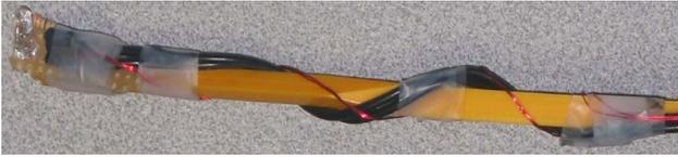
Figure 2. A calibration wand with a co-located sound and light source was constructed by attaching a microspeaker and a bright LED to one end of a long pencil.
