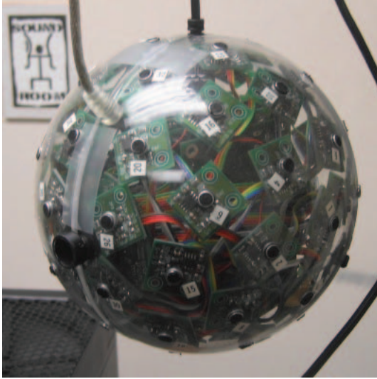
Fig. 1. An audio camera used for acoustic imaging – a 64-channel spherical microphone array with a video camera embedded.
