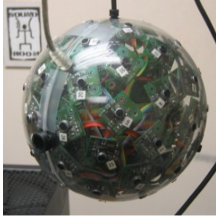
Fig. 7. A prototype 64-microphone array with embedded video camera. The array connects to the PC via a USB 2.0 cable streaming digital data in real-time.
