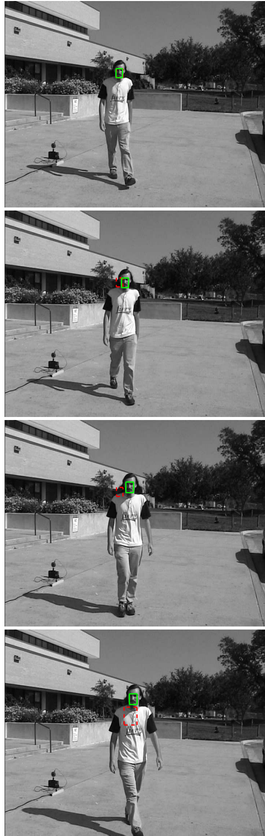
Figure 2. Sample frames in one probe video. The image size is 720x480 with the actual face size ranging roughly from 25x25 in to 40x40.
