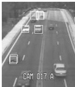
Figure 2. Results of the HOS-based vehicle detection scheme with dynamic background learning. Multiple boxes represent detection at different scales. Below each image, three values are given: they correspond to the number of vehicles detected, the number of vehicles present in the image, and the number of false matches, respectively. Vehicles that are much smaller than the training image are ignored in the calculations.
