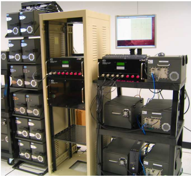
Fig. 2. The MeshTest testbed. The two racks on the left are the original twelve node testbed. The cart on the right is a smaller testbed that can support eight nodes.
