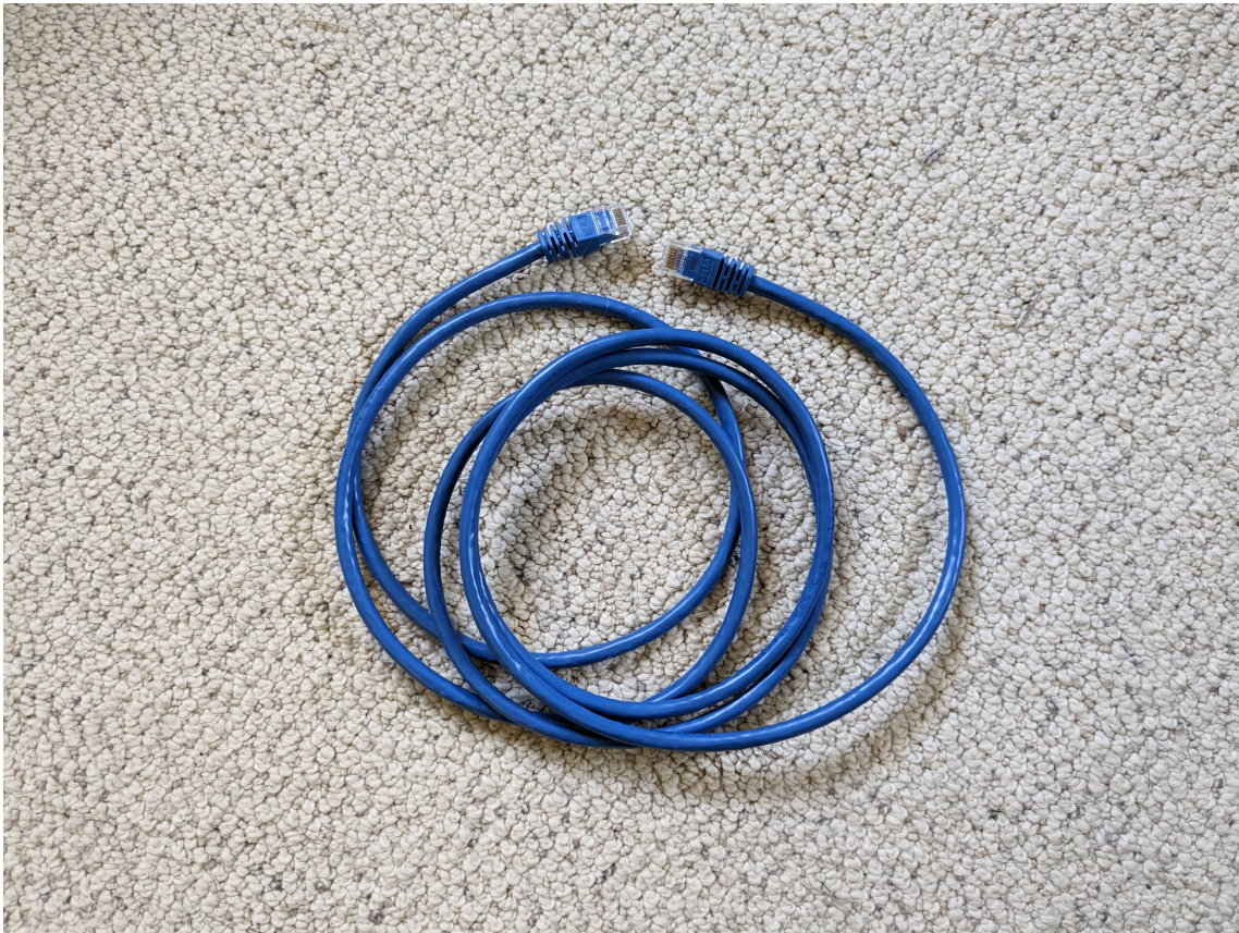
Figure 3.1: A Network Cable
