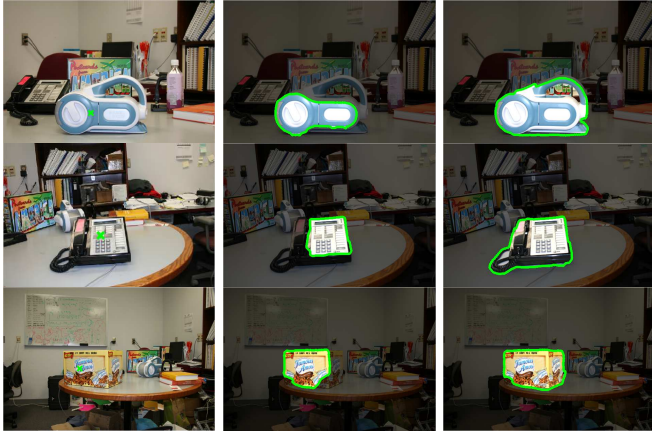
Fig. 7. Left: The frame of an image sequence captured with a moving camera. The fixation is shown by a green X. Middle: the segmentation using the boundary edge map as returned by martin et al.[9] using only monocular cues. Right: the segmentation using modified boundary edge map obtained by using motion cues to differentiate between internal and boundary edges.
