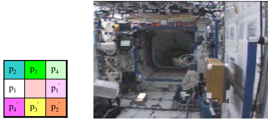
Fig. 1. (left) 3 \times 3 neighborhood with 4 center-symmetric pairs of pixels, (right) original space station image
