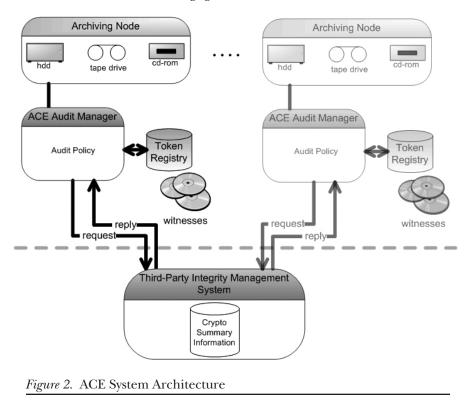
Figure 2 shows the overall ACE architecture assuming a distributed archiving infrastructure. A centralized archiving infrastructure will reduce to a single archiving node. The upper section represents the archive, the middle section contains the ACE-AM that is local to each archiving node, and the lower section represents the ACE-IMS, which is supposed to be outside the archive's domain and can support many different archives.
