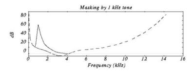
Experiment: Play 1kHz tone (masking tone) at fixed level (60 db). Play test tone at a different level and raise level until just distinguishable. Vary the frequency of the test tone and plot the threshold when it becomes audible.
