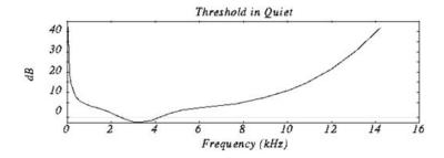
Experiment: Put a person in a quiet room. Raise level of tone at a given frequency until just barely audible. Vary the frequency and plot the results.
