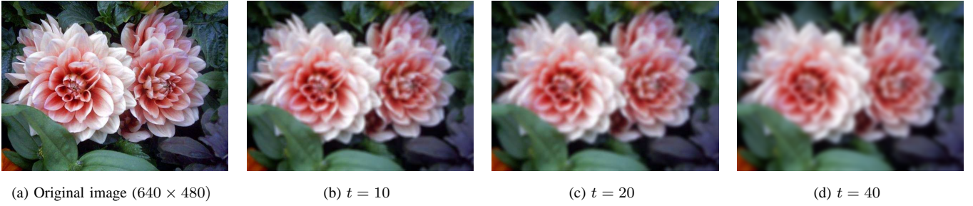
Fig. 2. Scale-space representation of a 2D image with increasing Gaussian kernel width.
