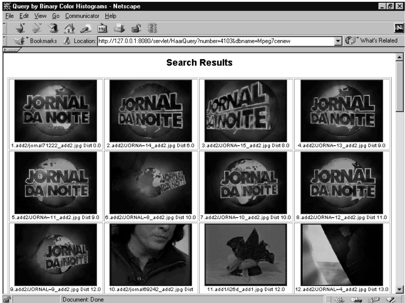
Figure 5: A sample result of image matching using binary Haar histogram descriptor
