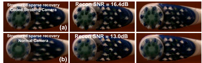
Fig. 14: Reconstruction results of toothbrush with upsampling factor U = 50 . Note that using CSC to capture periodic scenes allows us better reconstruction over using a normal camera.
