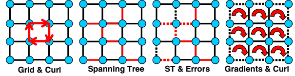
Figure 2. (a) Graph with pixels as nodes & gradients as edges. Curl is calculated along 2 \times 2 loops (b) Spanning tree edges in black (c) Gradient errors in dashed lines (d) Solid black lines and red curl loops have expander graph structure
