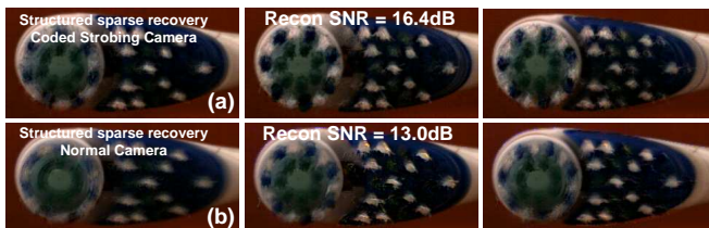
Fig. 14: Reconstruction results of toothbrush with upsampling factor U = 50 using structured sparse reconstruction and sparsity promoting super-resolution.
