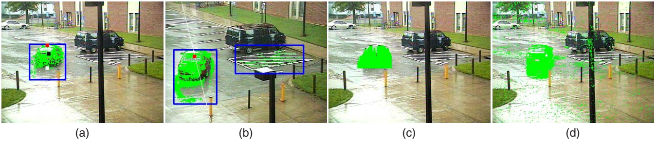
Figure 6: (a) Two-camera initial detection. Red square marks a sampled pixel while white square marks its base, computed using weak perspective model. (b) Single camera detection in the second view used to constrain stereo searches. Red square marks the conjugate pixel and white line is the associated epipolar line. (c) Two-camera final detection; specular region is removed since it lies below the base point in (a). (d) Single camera detection in the reference view for comparison.
