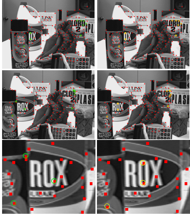
Figure 2. Tracking results of the original KLT (left column) and the proposed KLT (right column) using the time-reversibility constraint at the starting and ending frames. The green circled points on the left side differ significantly with the yellow circled points on the right side. It is easy to see that the new KLT keeps tracking those points well while the original KLT fails to track them.
