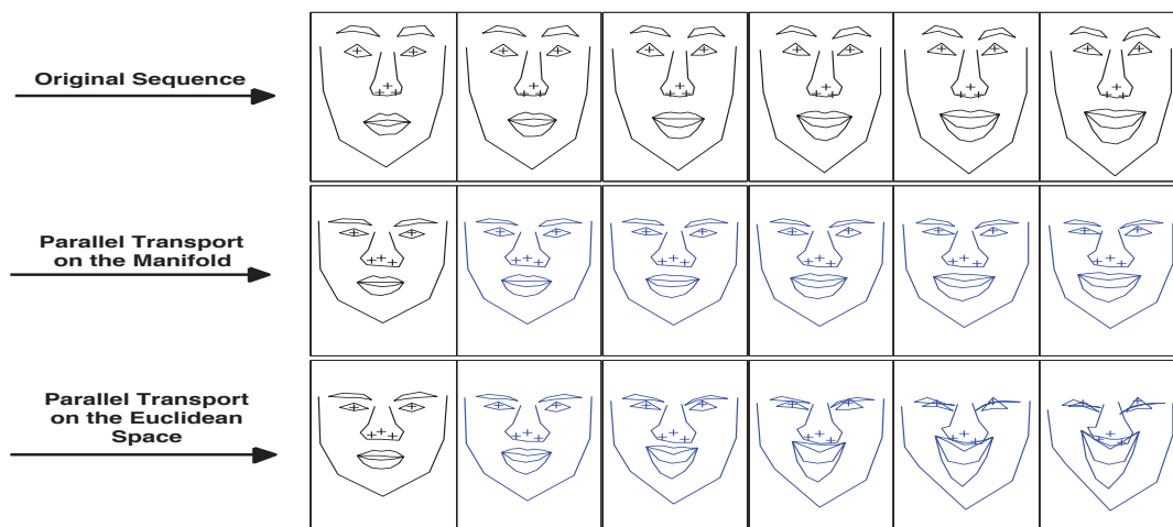
Fig. 7. Comparison between the results of parallel transport on the manifold versus that of Euclidean space. The first sequence (its tangent vector from the leftmost to the rightmost shape) is parallel transported to the face on the second and third row, and the new sequence is synthesized on the manifold (second row) and Euclidean space (third row).
