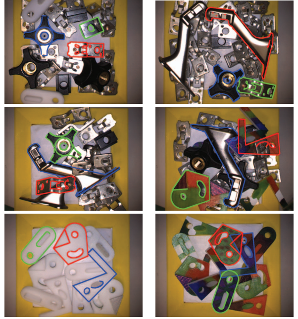
Fig. 11: Performance on real examples. The system detected and accurately estimated the pose for specular as well as textureless objects. Shown in these images are the top detector outputs for three different objects overlaid on top of the original images.
