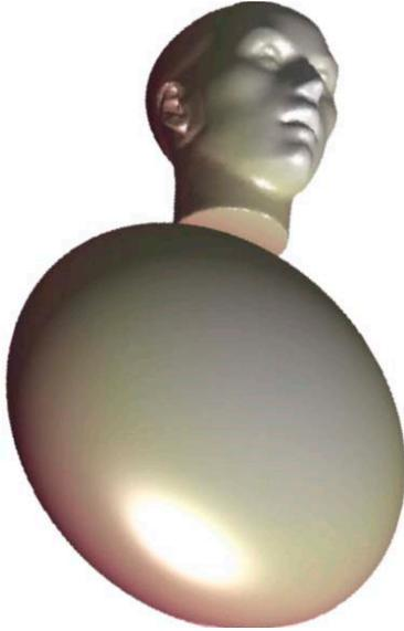
**Fig. 1.** A mesh of KEMAR used in our runs. The mesh has 54945 nodes and 109882 elements. The ellipsoidal torso dimensions are those in [2]. For the computations above 12 kHz the torso was meshed using a half ellipsoid, with the overall mesh having the same total number of nodes and elements.
