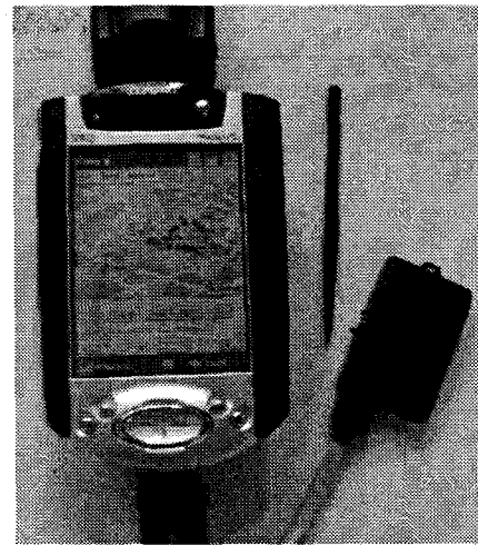
Figure 2. The mobile application eDiary on a Pocket PC equipped with the SoapBox as digital compass and with a GPS receiver.
