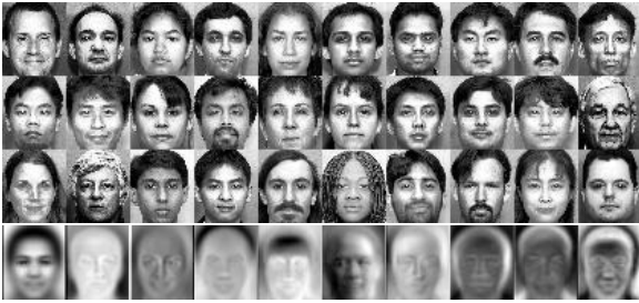
Fig. 4. II. The face gallery (upper) with image size 48x42. The top 10 eigenfaces (lower).
