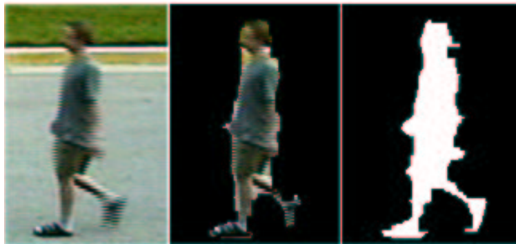
Fig. 2. Template types from left-to-right: original image, foreground template and binary template, of a walking person.
