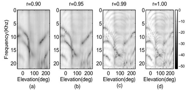
Figure 4: Frequency response of the time aligned and scaled LP residual for (a)  $r = 0.90$ , (b)  $r = 0.95$ , (c)  $r = 0.99$  and (d)  $r = 1.00$
