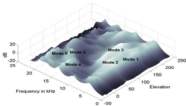
Figure 5: Frequency response of the 12<sup>th</sup> order all pole model for azimuth 0 as a function of different elevations. The six modes are approximately marked.
