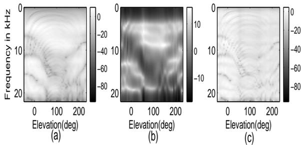
Figure 2: (a) The pre-emphasized HRTF image for right ear at azimuth  $0^\circ$ , (b) frequency response of a  $12^{th}$  order all-pole model and (c) the frequency response of the corresponding LP residual.
