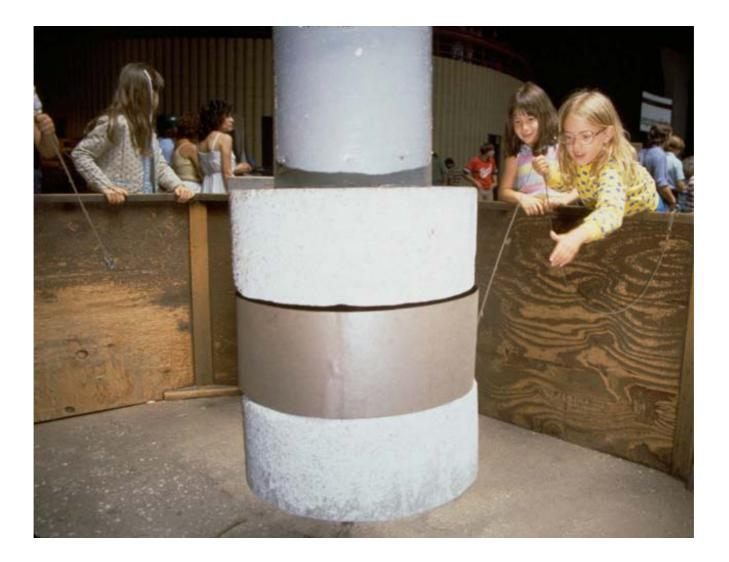
The giant 400-pound Resonant pendulum can only be given tiny tugs with weakly attached magnets on strings. A big swing can result if the tugs are timed with the swing of the pendulum.
