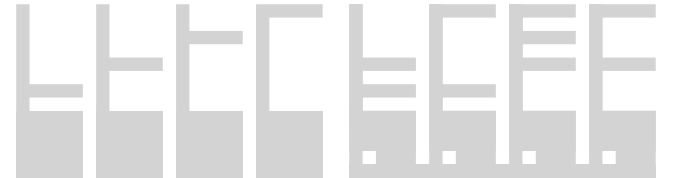
Figure 4: The set of polyominoes produced from the reduction from minimum set cover to smallest superpolyomino for the set \{\{1, 2\}, \{1, 4\}, \{2, 3, 4\}, \{2, 4\}\} .
