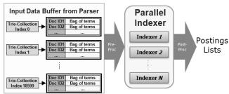
Fig. 6. Data Flow of One Single Run on Parallel Indexers
