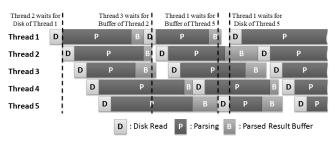
Fig. 8. Timing Sequence of Parallel Parsers
