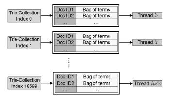
Fig. 5. Work Assignments among Multiple Indexer Threads
