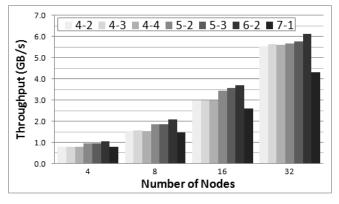
Fig. 16. Optimal Number of Parsers and Indexers on Cluster in Distributed Model
